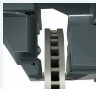
Simultaneous dual-face turning of disk brake
