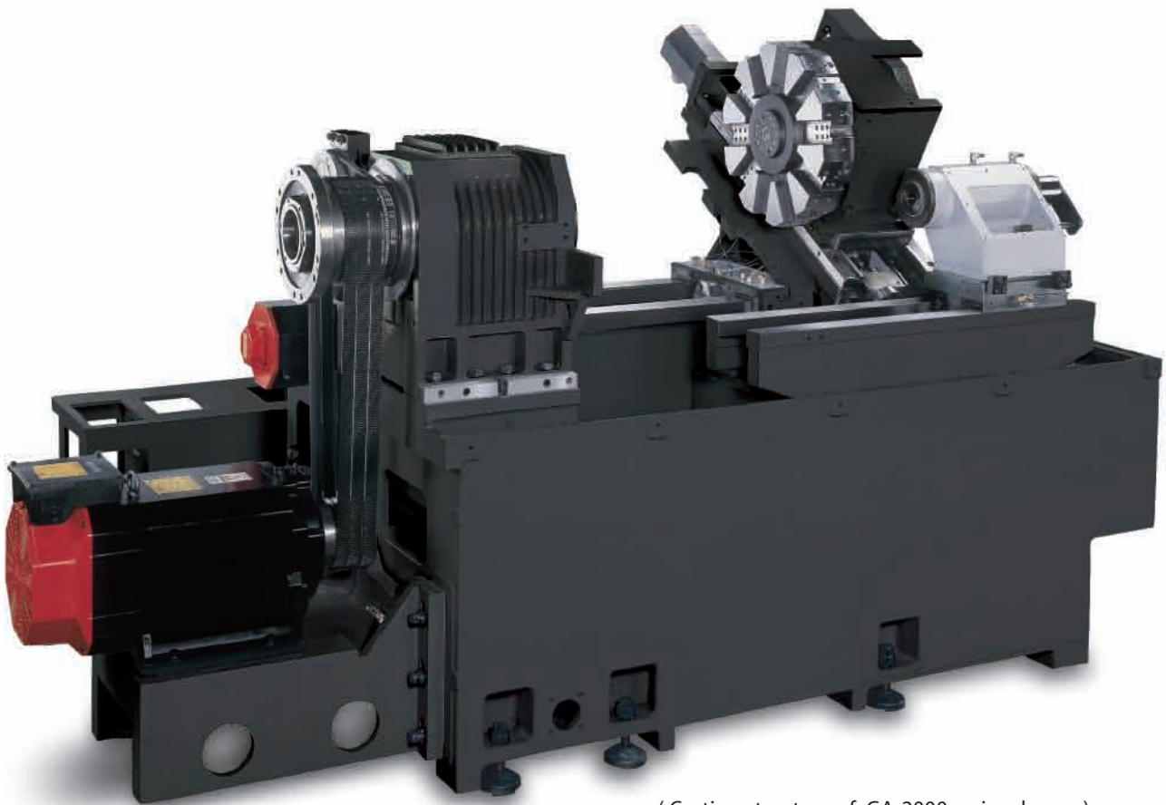
( Casting structure of GA-2000 series shown. )
