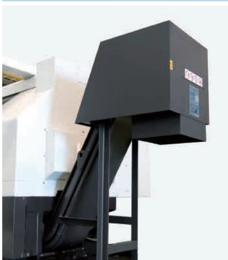
Right discharge chip conveyor
